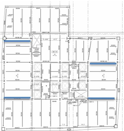
Figure 4 | Location of Composite Beams (S108)
